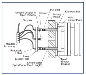
This setup is designed for custom molders who use a variety of injection molds with different knockout patterns and ejector strokes.
