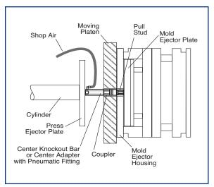
For small presses with a center knockout, replace the cylinder bolt (if present) with a Center Knockout Bar and FasTie Coupler.
